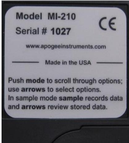
Sensor model number and serial number are located on a label on the backside of the handheld meter.
